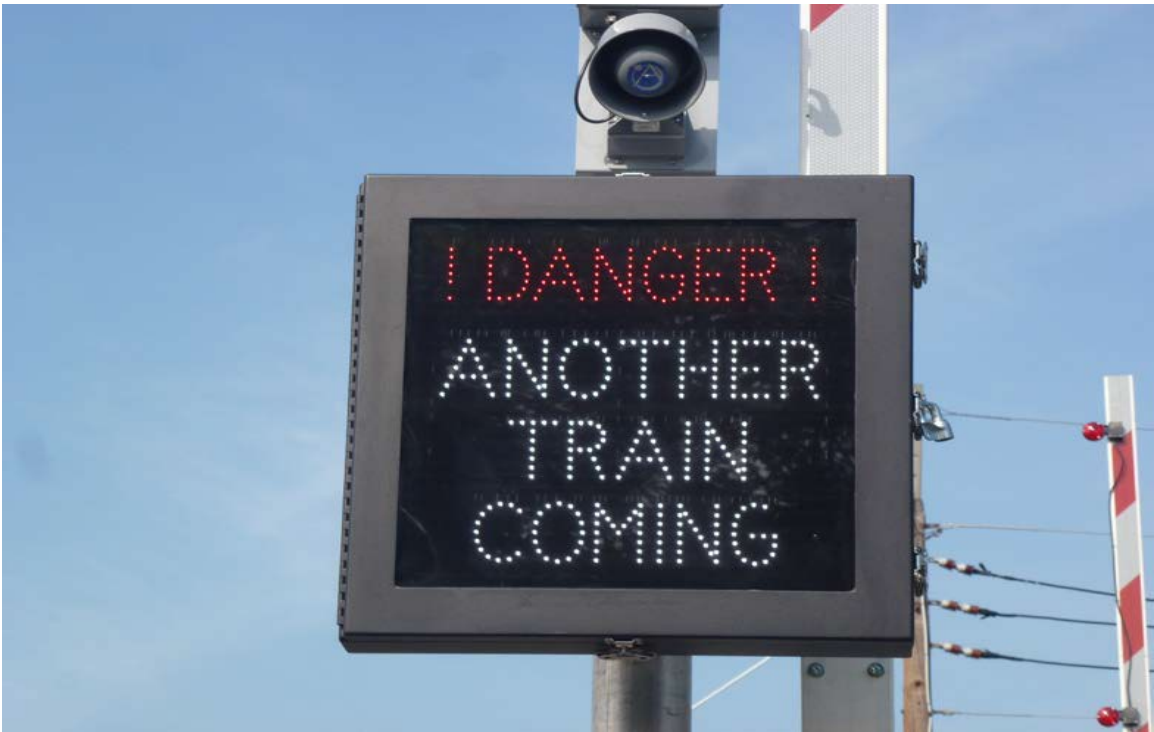
Figure 3. Example of a second train warning system at a crossing in Garfield, NJ Image Credit: Volpe Center
