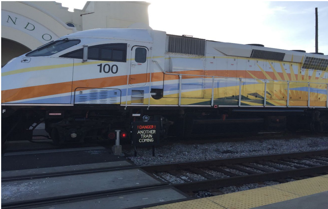
Figure 4. Example of a second train warning system at a station crossing in Orlando, FL Image Credit: Volpe Center
