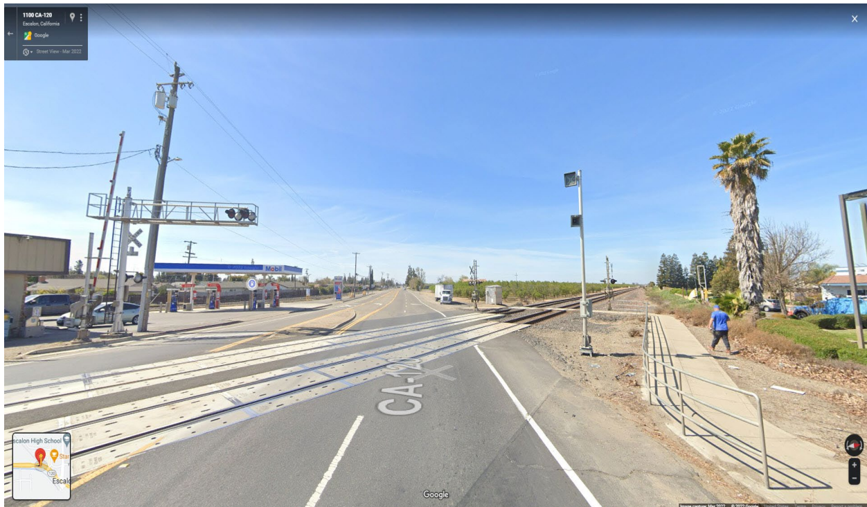
Figure 1. Example of a wayside horn at a grade crossing in Escalon, CA from Google Street View
