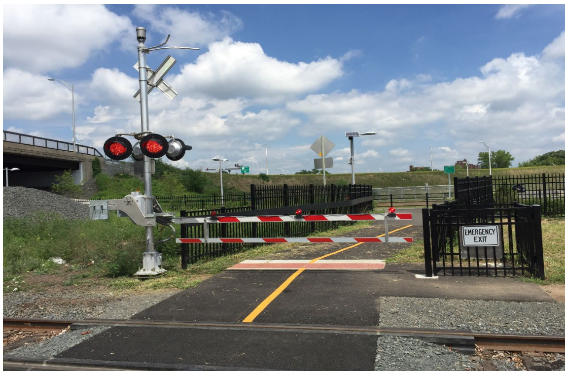
Figure 2. Example of a hinged pedestrian gate skirt at a pathway crossing in New Britain, CT Image Credit: Volpe Center
