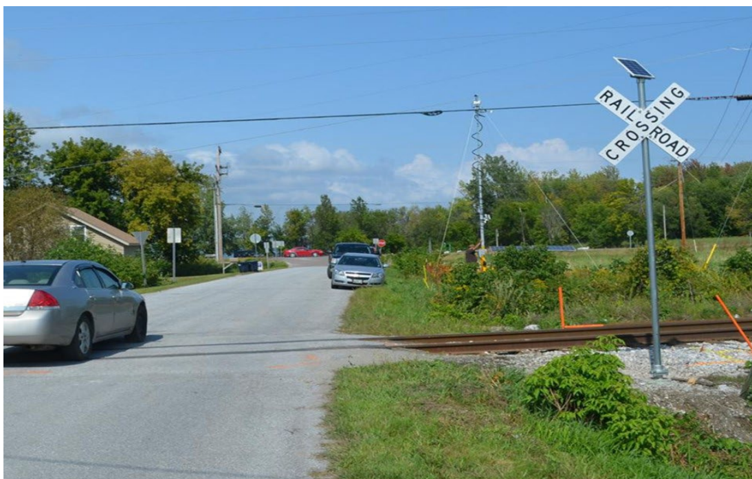
Figure 2. Example of LED-enhanced Crossbuck sign (R15-1) at a grade crossing in Swanton, VT Image Credit: Volpe Center
