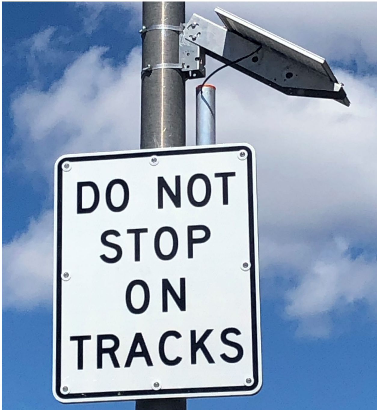
Figure 3. Example of LED-enhanced DO NOT STOP ON TRACKS sign (R8-8) at a grade crossing in Belmont, MA Image Credit: Volpe Center
