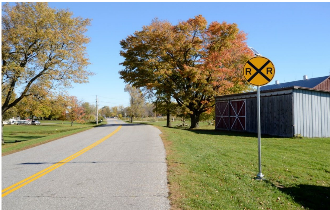
Figure 1. Example of LED-enhanced Advanced Warning sign (W10-1) at a grade crossing in Swanton, VT Image Credit: Volpe Center
