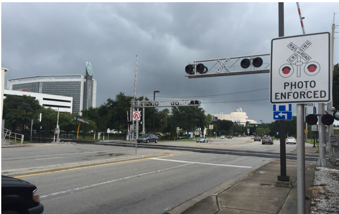
Figure 2. Example of photo enforcement signage at a grade crossing in Orlando, FL Image Credit: Volpe Center
