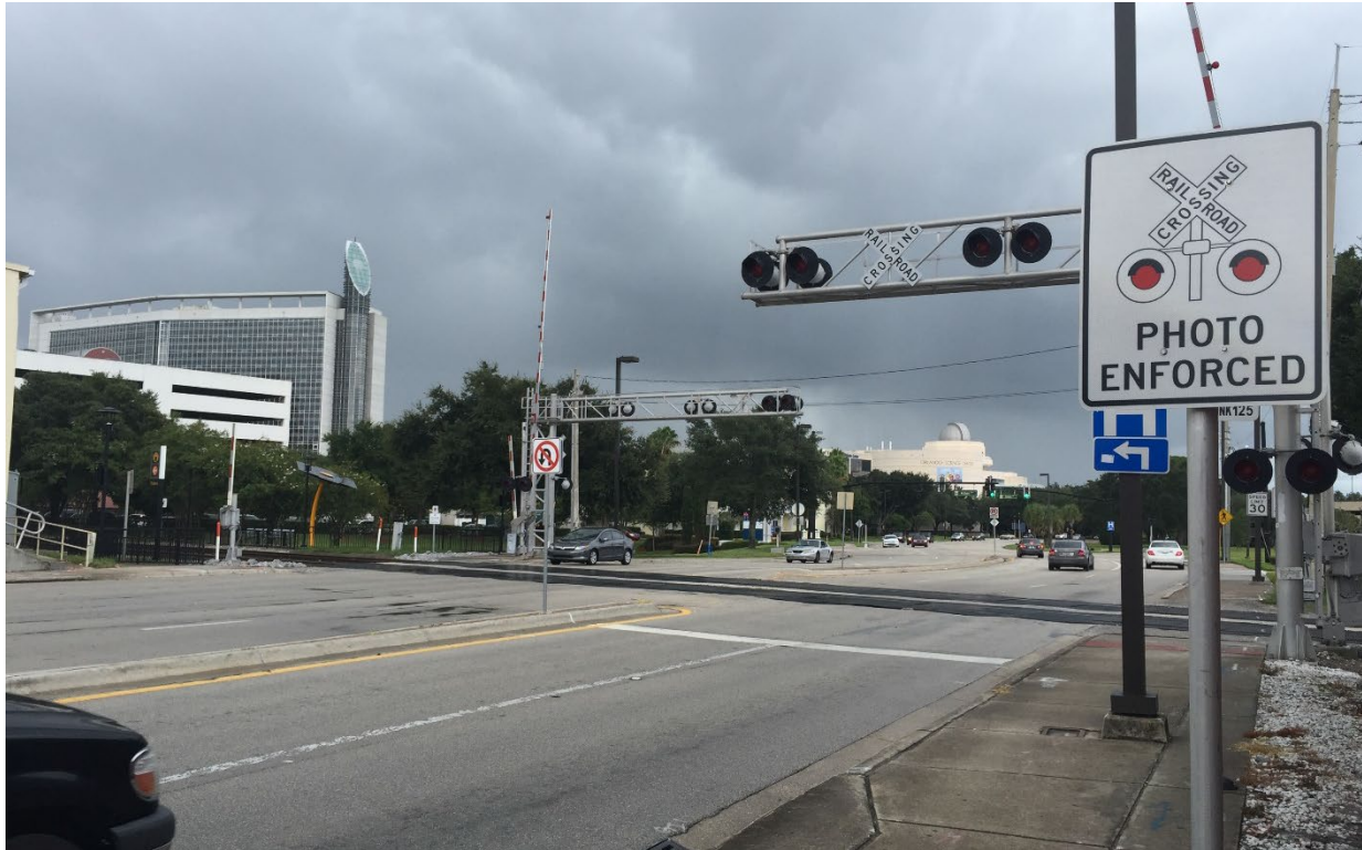
Figure 2. Example of a photo enforcement signage at a grade crossing in Orlando, FL Image Credit: Volpe Center
