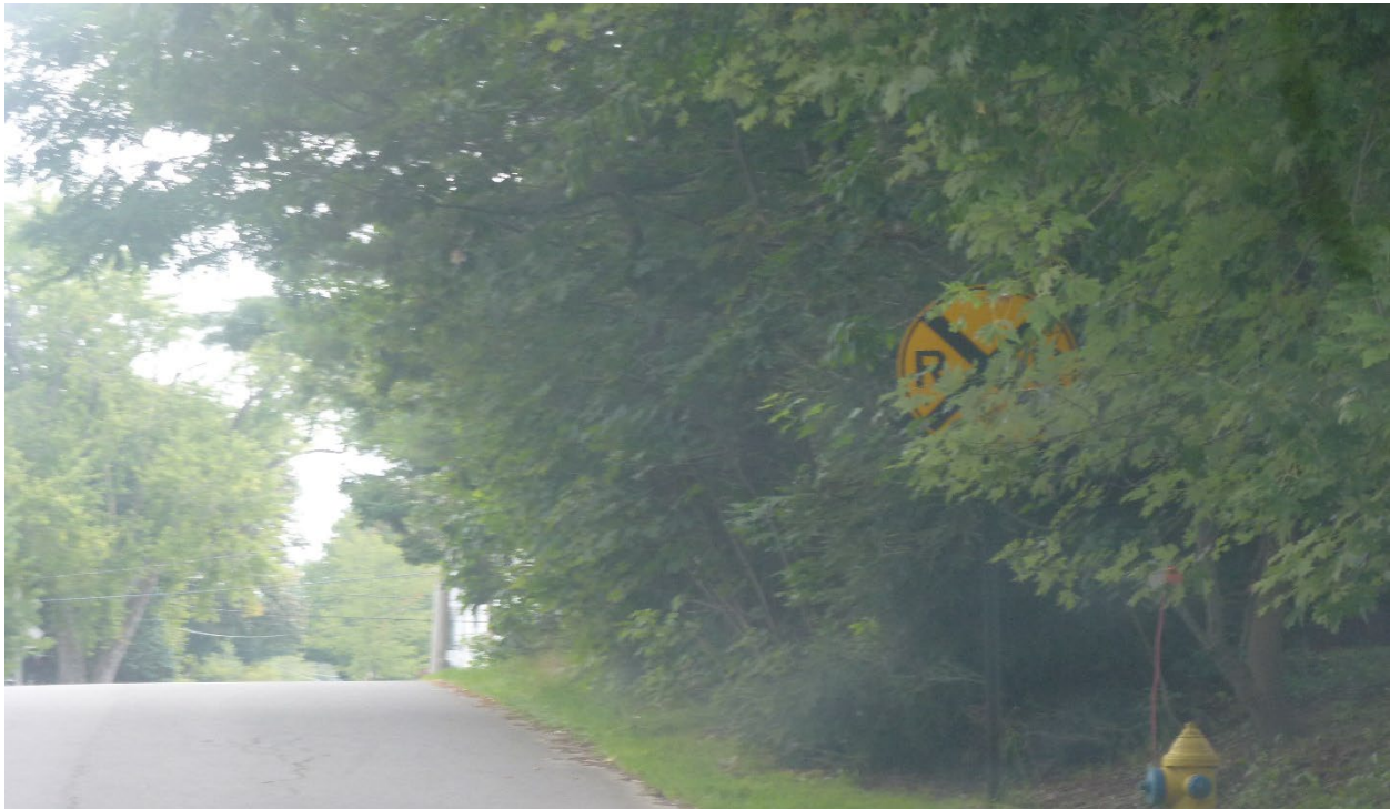
Figure 2. Example of vegetation obstructing advanced warning signage on approach to a crossing in Brunswick, ME Image Credit: Volpe Center
