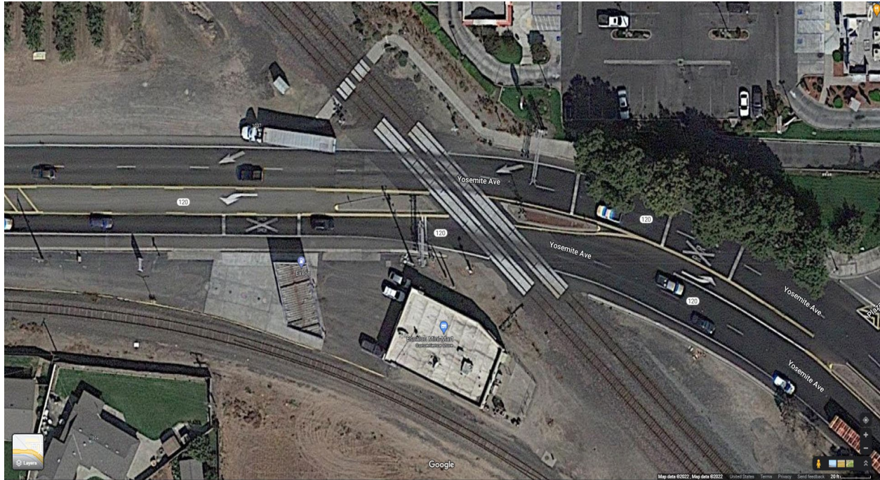
Figure 1. Example of crossing alignment adjustment for non-motorized users from Google Satellite View
